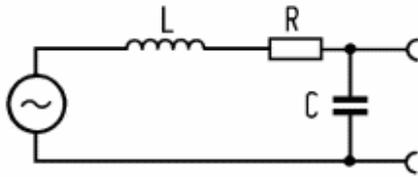
containing an ohmic resistance, a capacity and an inductivity.
